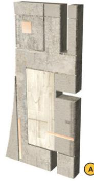
Sculptural precast curved wall, one of four segments shown. Each wall segment is 10' high, 10" thick and up to 10' wide. Final sculptural configuration will have a specially engineered set of shop draw-
