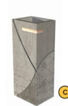
The Sculptural biofiltration chambers are detailed to ensure the proper placement and function of the packing media. The nominal dimensions are 2' wide and 1.5' in depth with 5' and 3' height elements.
