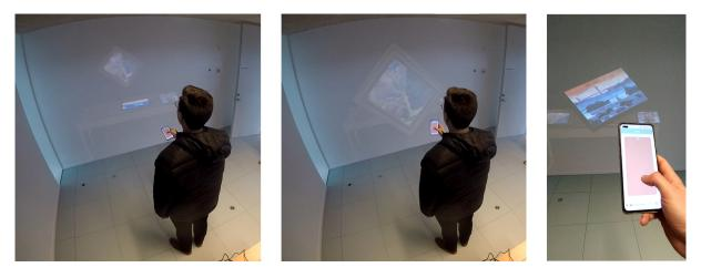
**Figure 6** In the 3D setup, the participant uses a smartphone to control a cursor on the screen. It can be used to pick up, move, and tilt the virtual paintings. The first two images are video stills from the experiment. The third is a staged closeup.
